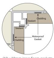
(12 x 10mm inner foam gaskets optional, alternative sealant option)
