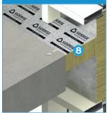
SIDERISE CW-FS perimeter barriers are market leading fire, smoke and acoustic seals for use within curtain walling. The range includes different options to suit required fire ratings and/or acoustics performance.
