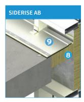
SIDERISE AB are acoustic barrier overlay materials for use above the perimeter barrier firestop. Different grades are available to suit acoustics performance required.
