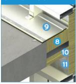
SIDERISE CVB is a high mass closure normally incorporated beneath the perimeter barrier firestop and located to maximise the air gap and create a "twin mass" system.
